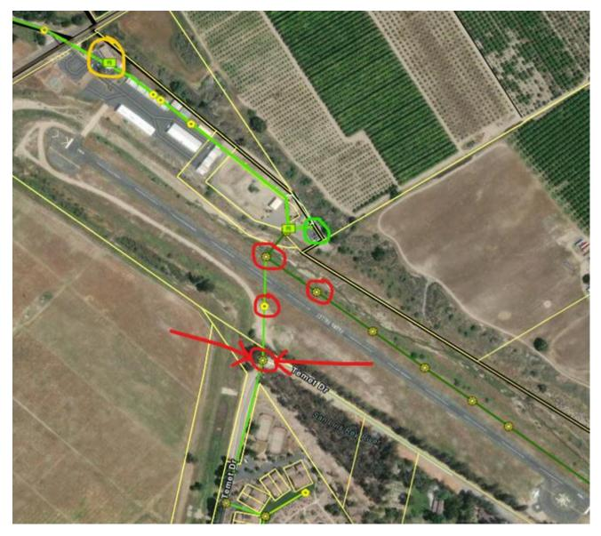
The two red arrows highlight the maintenance hole that will likely cause an issue or result in a spill (SSO). This is the primary maintenance hole to monitor.
